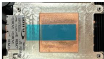
Figure 3: Heatsink 2, with PTM7950 on top
