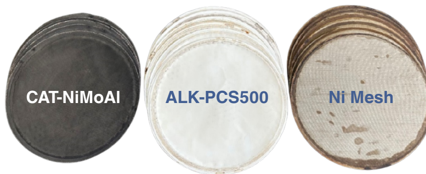
Disassembled electrolyzer after 5 months of stable operation
