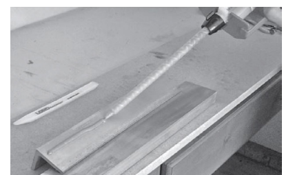
Figure 7. Position and dispense adhesive.
