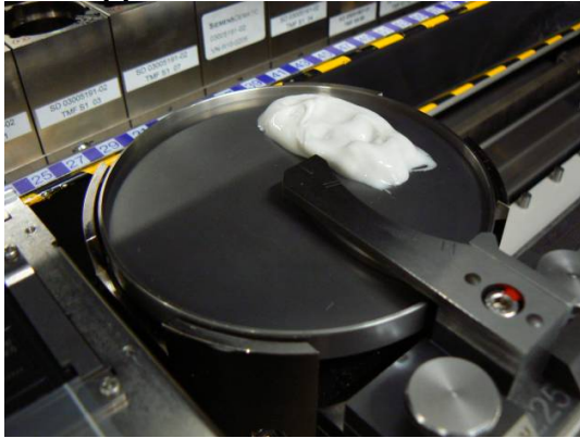
Flux Dispensed in Rotating Application Tray
